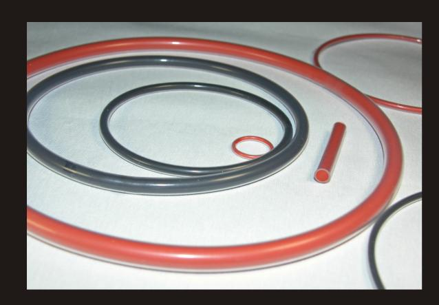
FEP encapsulated O-ring can resist the erosion of almost all the chemicals. It can be used in a wider range of temperature with good compression property, friction-resistance, seal endurance and longer sealing life. It is mainly used in pump, valve, reactor, mechanical seal filter, pressure container, heat-exchange container, boiler, flange, gas compression motor etc..
